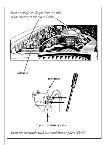
An easy way to find it is to follow the positive battery cable. You will see a small wire and the positive battery cable. Cross the two with a screwdriver or pliers. This cranks the engine.
