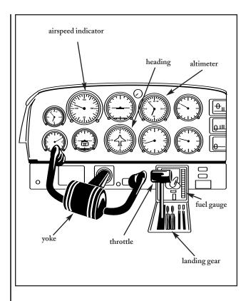
THROTTLE. This controls airspeed (power) and also the nose attitude, or its relation to the horizon. It is a lever between the seats and is always black. Pull it toward you to slow the plane and cause it to descend, push it away to speed up the plane and cause it to ascend. The engine will get more or less quiet depending on the direction the throttle is moved.
