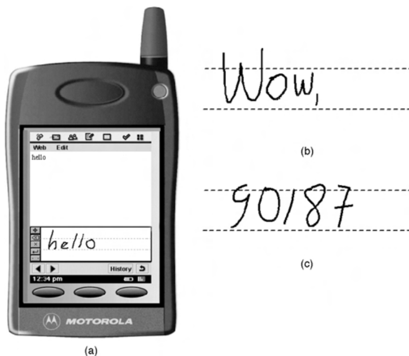
FIGURE 42.38 Word-based text input method for mobile devices. In (a), a user interface prototype. In (b), an image of the mixed-case word “Wow,” where relative size information can be used for distinguishing among the letters in the “Ww” pair. In (c), an image of the digit string “90187” where ambiguity in the identity of the first three letters can be resolved after identifying the last two letters as digits.
