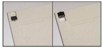
Your 3.5-inch floppy disk has a plastic slider that is used to write-protect the disk. When it's down you can write to the disk, when it's up the disk is write-protected.
